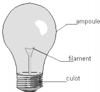
ampoule + filament + culot = LAMPE
